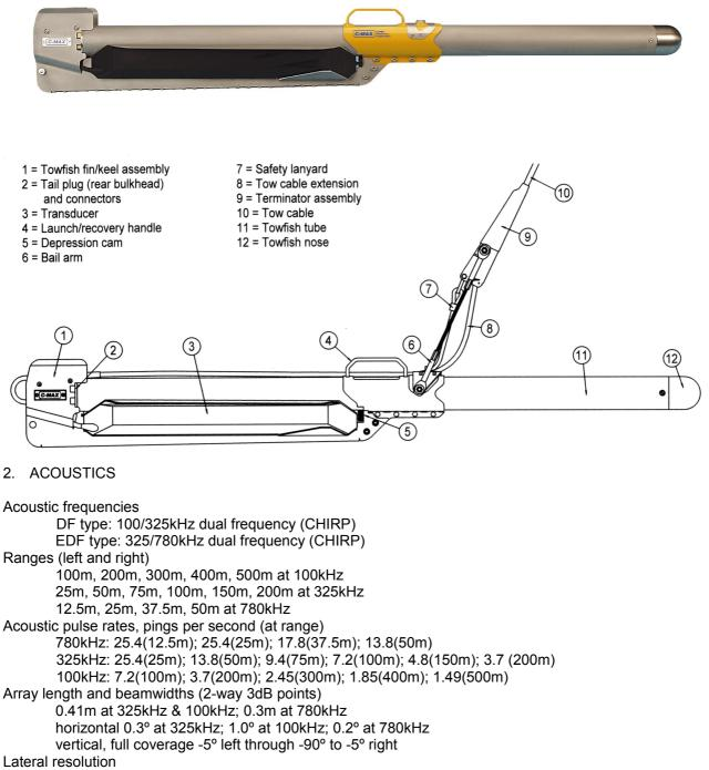
18mm at 780kHz; 39mm at 325kHz (18mm at 25m range); 78mm at 100kHz
